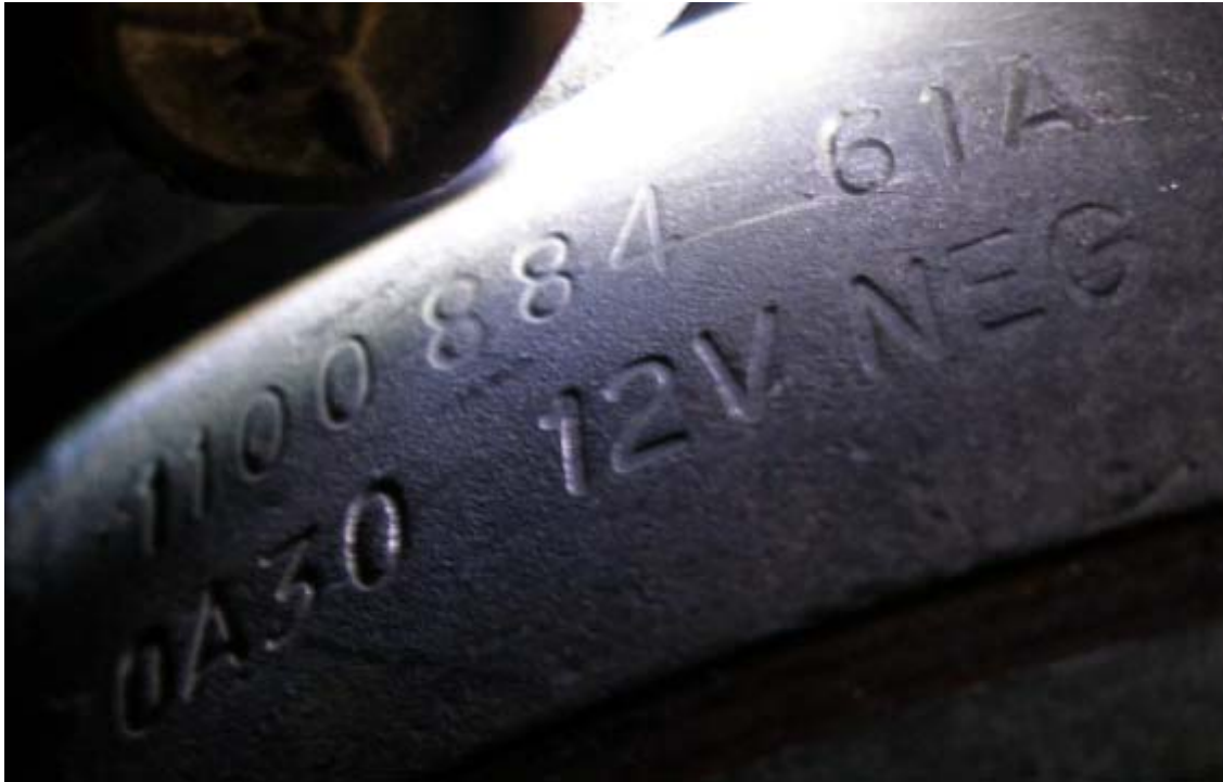
Alternator Code - 1100884 (Original for Air Condition cars) 0A30 – January 30 th Casting Date.
