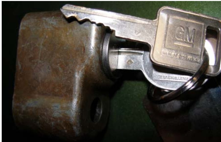
Correct Coded Original Keys The "J" key for 1970 Ignition & Doors The "K" key for 1970 Glove box & Spare tire Lock
