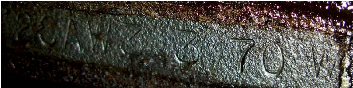
Rear Axle Code – 2CAW 3 3 70 W CAW – Positraction 3.08 ratio 4-Speed Automatic 3 – Month, March 3 – Day, 3 rd 70 – Year, 1970 W – Plant, Warren Plant
